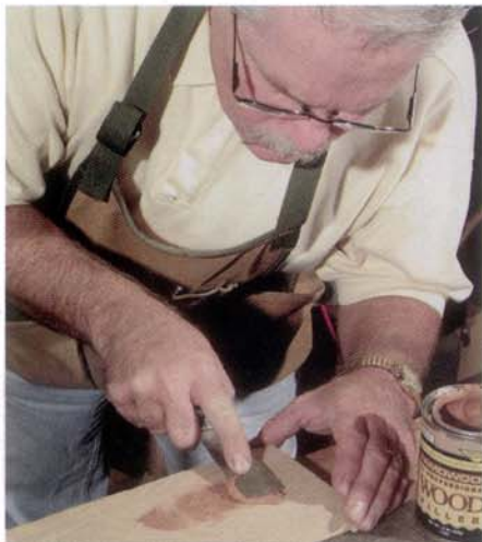
When repairing cracks or defects, press the wood filler firmly into the damaged area with a putty knife.
