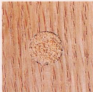
Sawdust in this solvent-based putty resulted in a coarse-textured patch that looked bad and absorbed too much finish.
